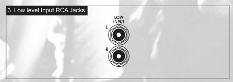
These inputs are for signal cables from the source. Always use high quality, shielded RCA cables.
